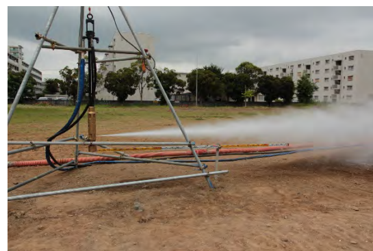
Fig. 18. Newly-developed small and light-weighted jet-grouting machine
