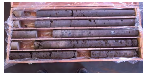
Fig. 21. Collected specimen of solidified clayey soil after modified working procedure
