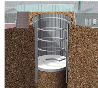
1. Installing piles to form the cylindrical wall
