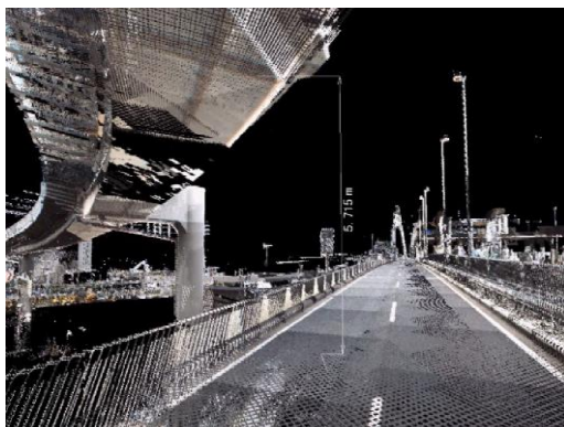
Figure 5 Clearance check in the space by point cloud data
