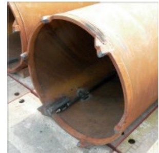
Photo 8. Tubular Piles with pile toe ring bits
