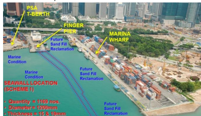
Fig. 2. Proposed Seawall & Future Reclamation
