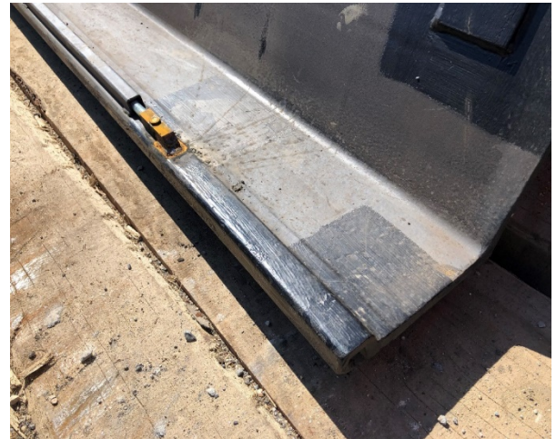
Fig. 5. Non-declutching Sensor and Cable Conduit
