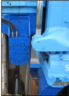
Picture 4 Water Jetting System
