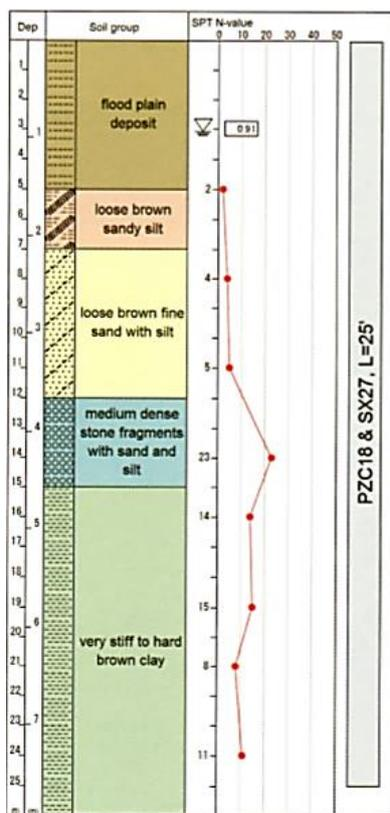
Fig. 4. Soil Conditions and Sheet Pile Location
