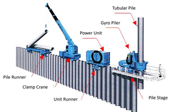
Fig. 8. Concept of GRB (Giken Reaction Base) System
