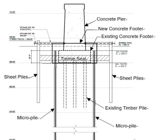
Fig. 3. Cross-section of Cofferdam and Pier Foundation (Source: Richard Goettle Inc.)
