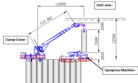
Fig. 12. Pipe Section Supplied by Clamp Crane
