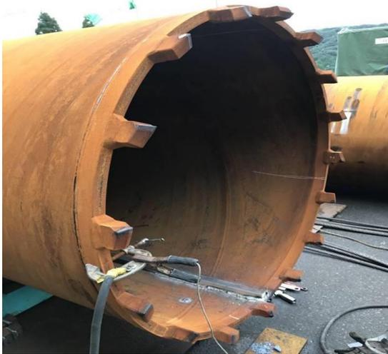
Fig. 10. Cutting Shoe of Pipe Pile (Sacrificial)
