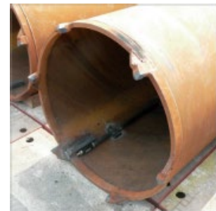
Photo 8. Tubular Piles with pile toe ring bits
