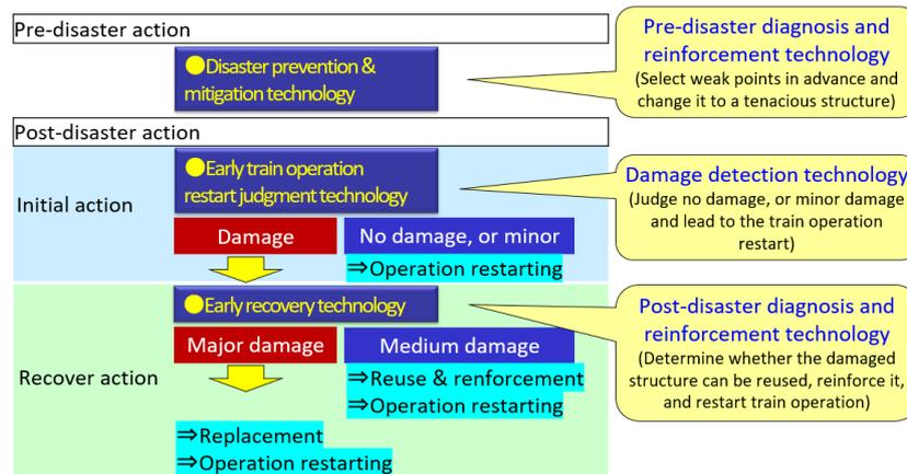
Fig.6. Railway disaster countermeasures (pre- and post-disaster actions)
