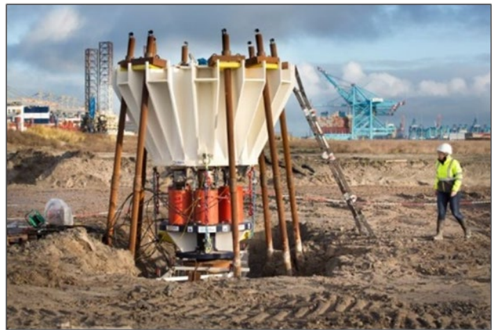
Fig. 5. (b) Axial load test set-up
