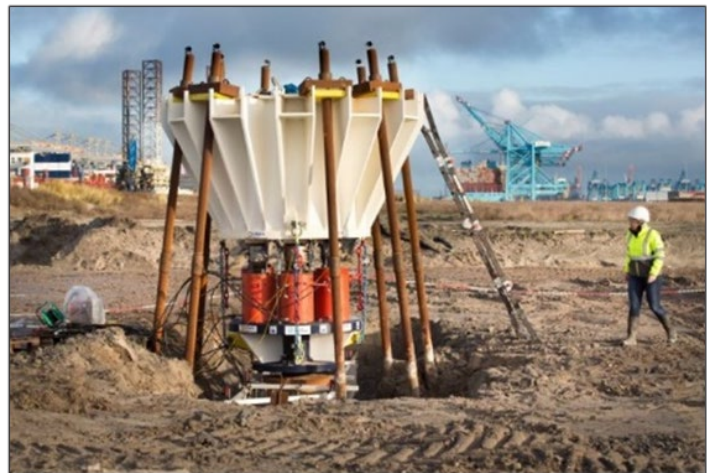
Fig. 5. (b) Axial load test set-up
