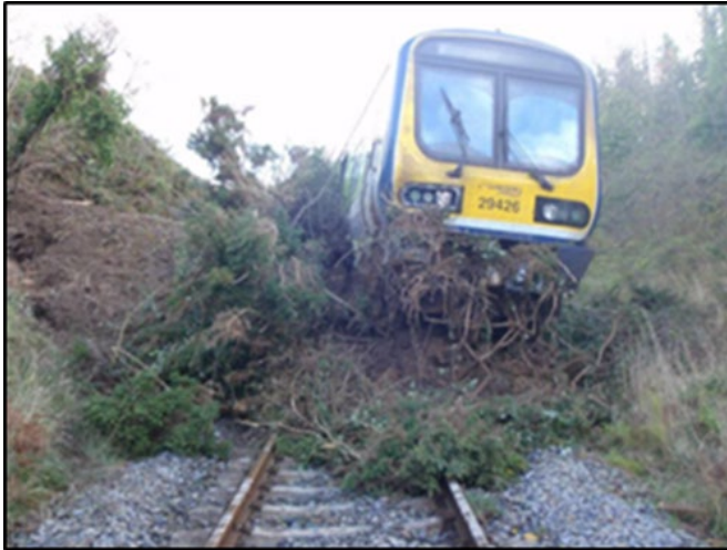
Fig. 3. (a) Example of shallow translational slip causing train derailment
