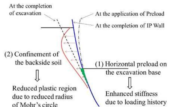
Fig. 13. Mechanisms of smaller deformation of Preload Retaining Wall (Ishihara et al. (2015))
