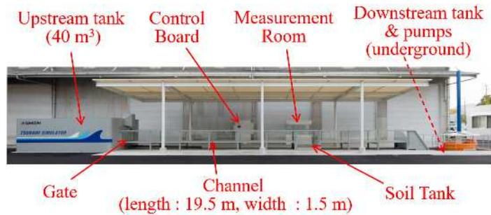
Fig. 17. Experimental apparatus to simulate tsunami (after Ishihara et al. (2018))
