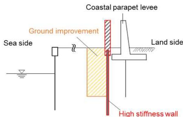
Fig. 1. Cross section of the seawall seismic reinforcement
