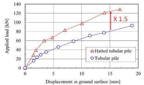
Fig. 4. Results of full-scale horizontal load tests (after Ishihara et al. (2016))
