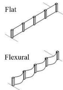
Fig. 19. Shapes of wall members (after Toda et al. (2021))
