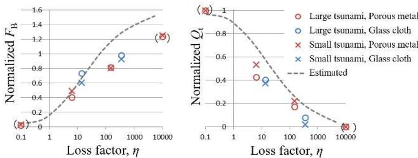
Fig. 18. Experimental results in comparison with estimated results (after Suzuki et al. (2016))
