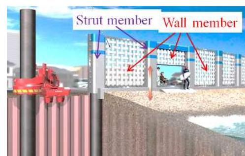
Fig. 15. Basic structure of Implant Barrier (after GIKEN (2023))
