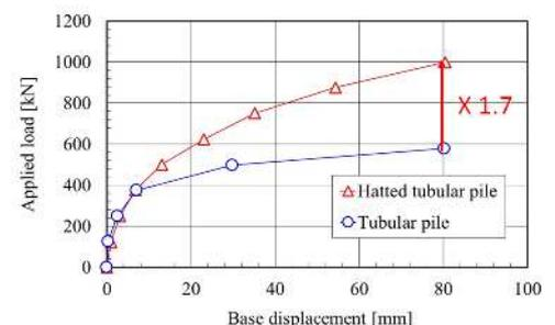
Fig. 3. Results of full-scale vertical load tests (after Ishihara et al. (2016))
