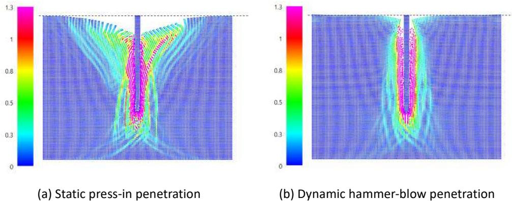
Fig. 4. Numerical simulation of sheet pile penetration into ground. Maximum shear strain distribution for the static and dynamic penetration cases.
