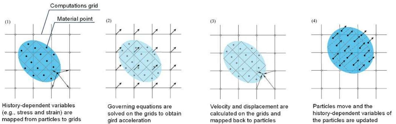
Fig. 2. Numerical algorithm of Material Point Method
