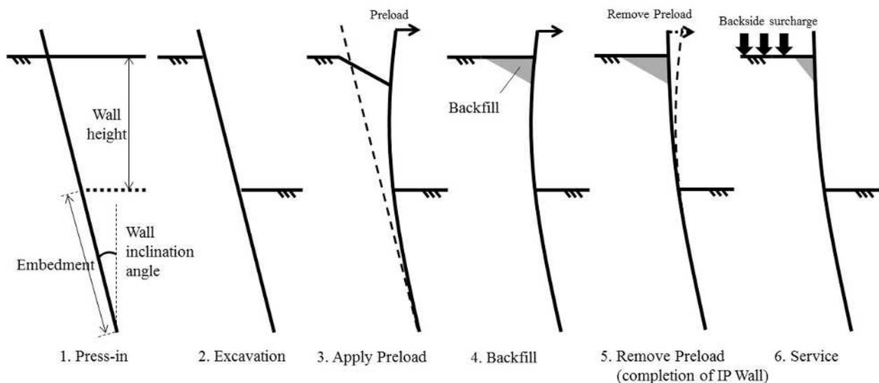
Fig. 11. Construction procedure of Preload Retaining Wall (Ishihara et al. (2015))
