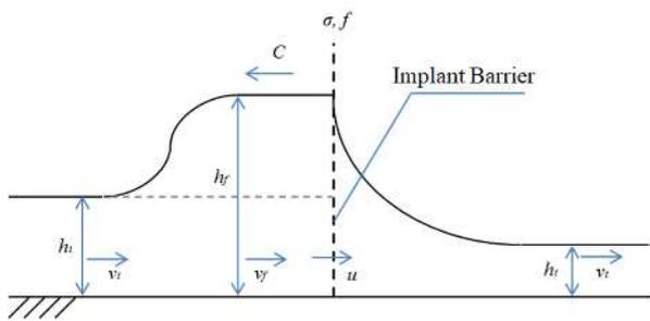
Fig. 16. Theoretical approach for Implant Barrier (after Suzuki et al. (2016))
