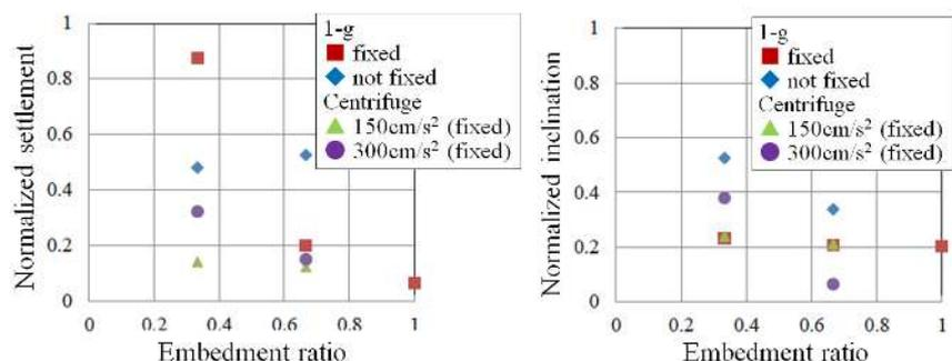
Fig. 7. Experimental results on the effect of square sheet pile wall on reducing settlement and inclination of house due to liquefaction (Kato et al. (2014))
