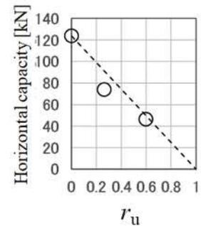
Fig. 9. Horizontal capacity vs.  $r_u$  (after Toda et al. (2023))
