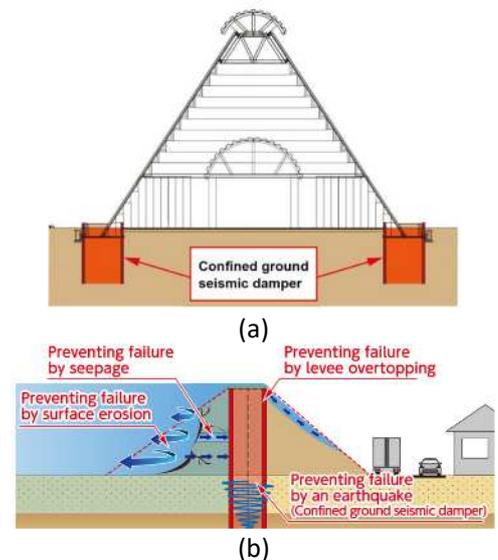
Fig. 5. Application examples of Confined Ground Seismic Damper (GIKEN (2023))
