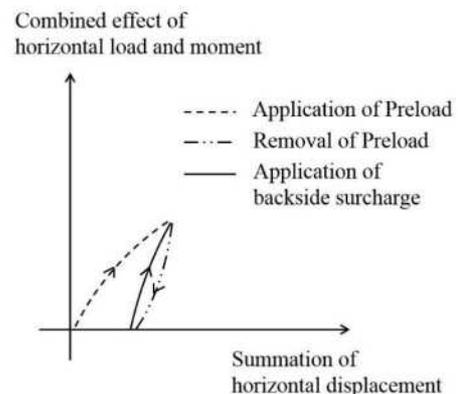
Fig. 14. Conceptual diagram for design of Implant Preload Wall (Ishihara et al. (2015))
