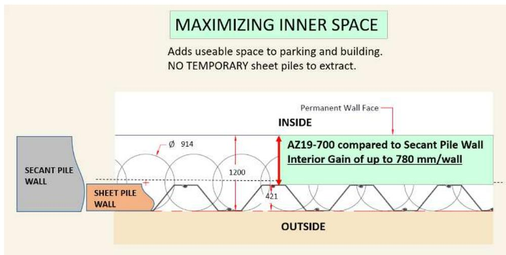
**Fig. 1. Larger inner space with sheet pile wall than with secant pile wall**
