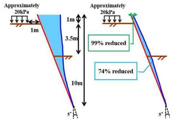
(a) Slanting wall (b) Preload Retaining Wall
