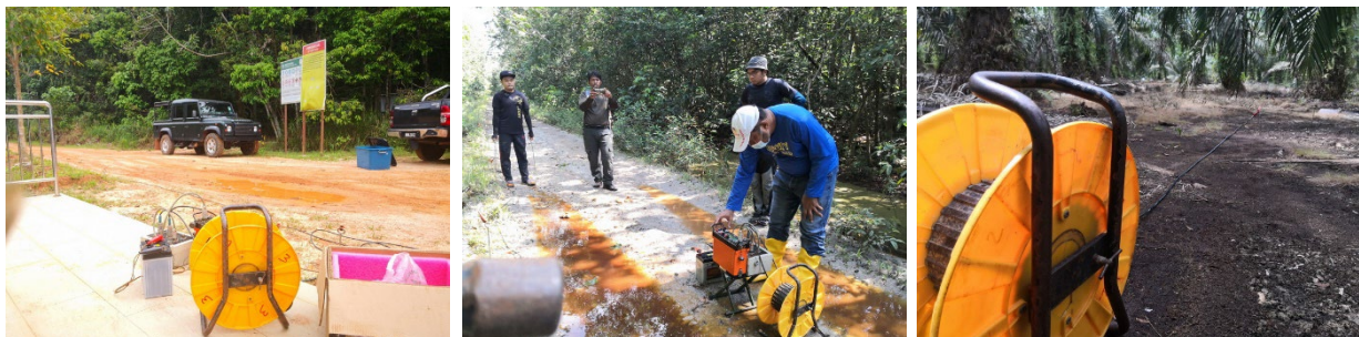
Fig. 1. Resistivity line survey conducted of few locations inside North Ayer Hitam State Forest Reserve, Muar, Johor
