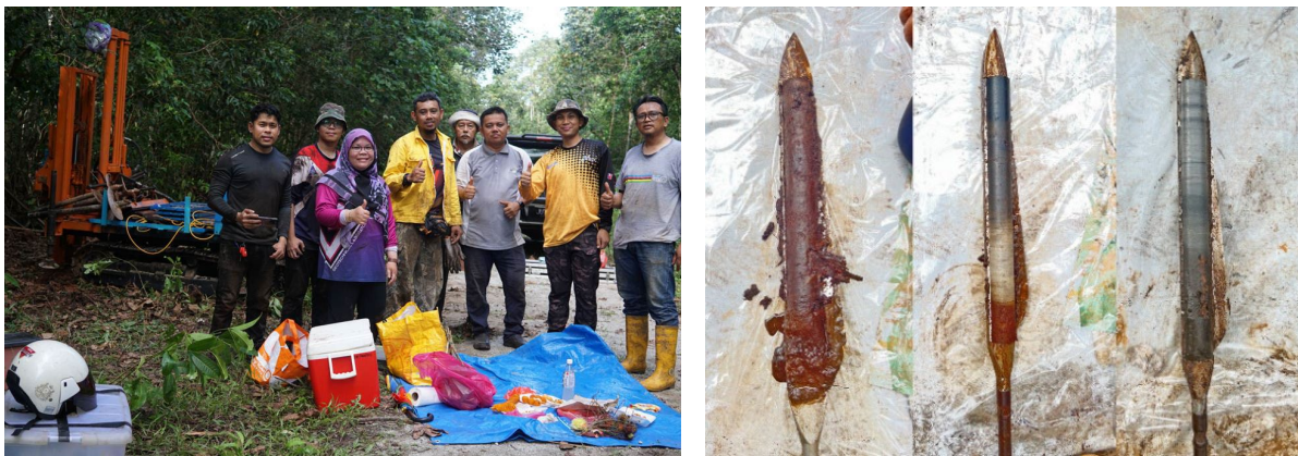
Fig. 3. An expedition by UTHM team to assess depth of peat in the forest (left) and the peat sampling made using a peat sampler during the expedition (right)
