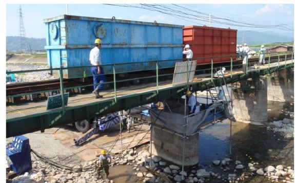
Fig. 2. View of Static loading test by water tank [2]
