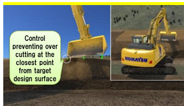
Fig. 16 Bucket control point and closest distance control
