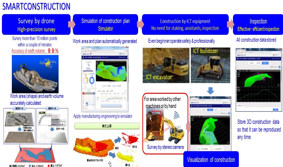
Fig. 3 New process realized by SMART CONSTRUCTION
