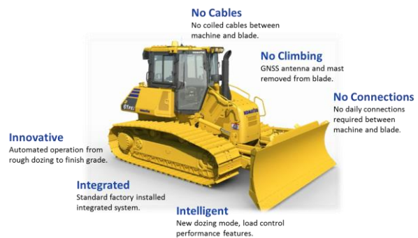
Fig. 9 Komatsu ICT Bulldozer
