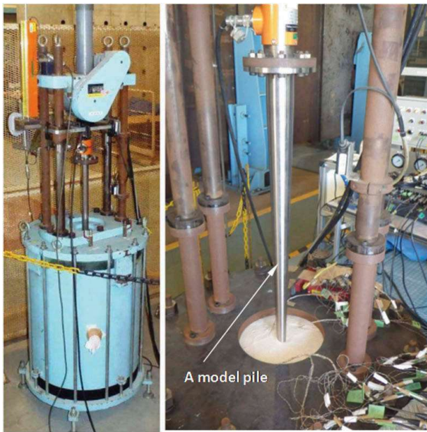
Figure 2. Photographs of the experimental apparatus (left) and the tapered model pile under testing (right).
