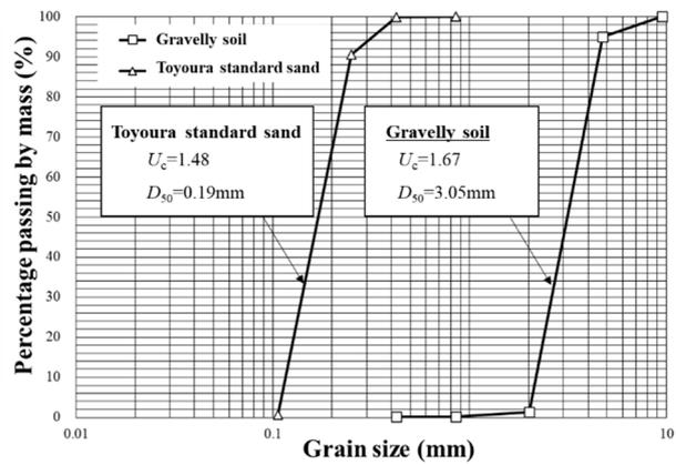
Fig.4 Grain size accumulation curve of the ground material used in the experiment
