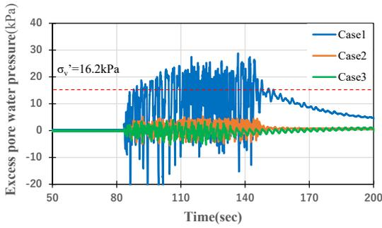
Fig.7 Excess pore water pressure at point p1
