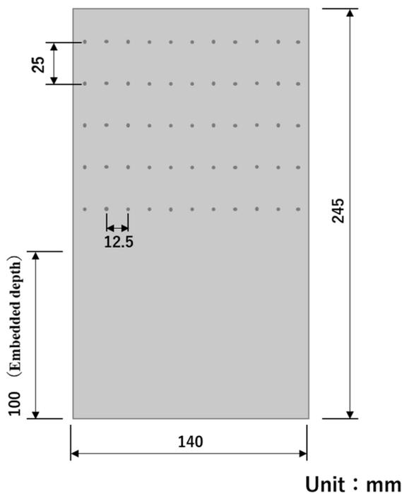
Fig.3 Hole arrangement of permeable steel sheet pile
