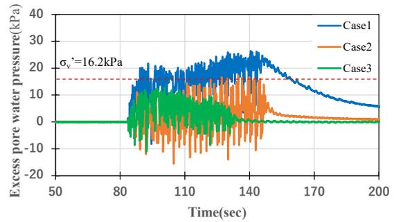
Fig.10 Excess pore water pressure at point p4
