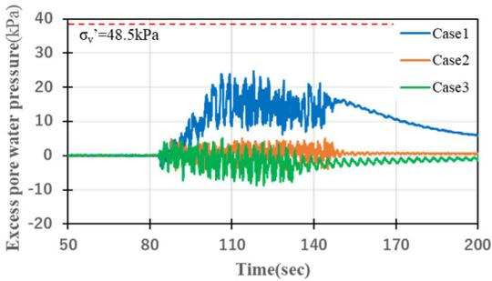
Fig.9 Excess pore water pressure at point p3
