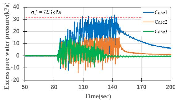
Fig.11 Excess pore water pressure at point p5
