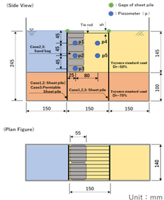
Fig.2 Experimental model for the study case
