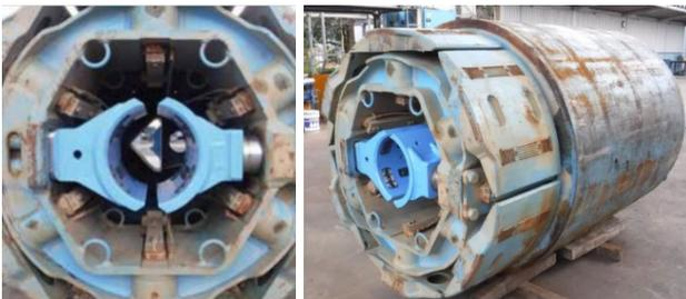
Fig.8 Driving attachment (pile follower) with a built-in small chuck
