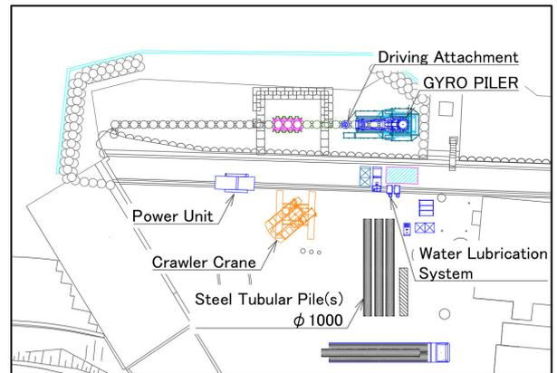
Fig.19 Plan view (Tubular pile)
