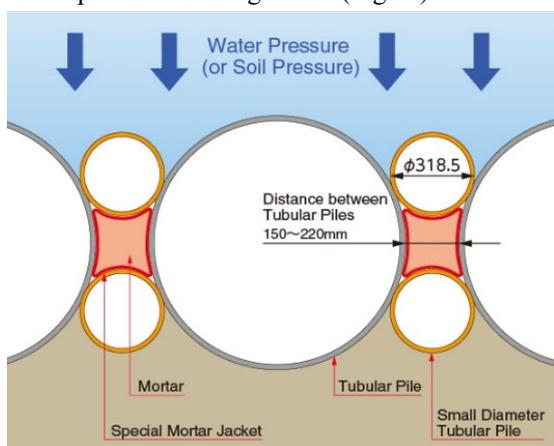
Fig.14 Waterproofing method
