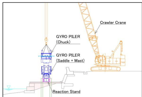
Fig.21 Cross section
