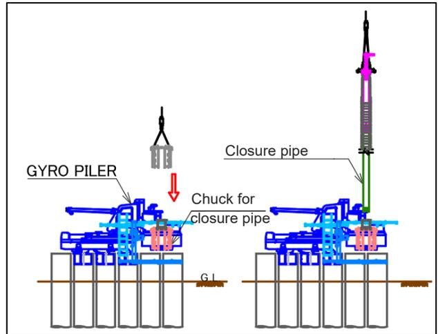
Fig.10 Installation of closure pipes and mortar jacket (Chuck for closure pipe installation)
