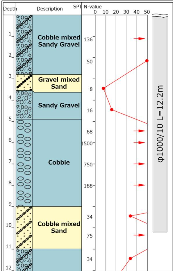
Fig.4 Borehole log
