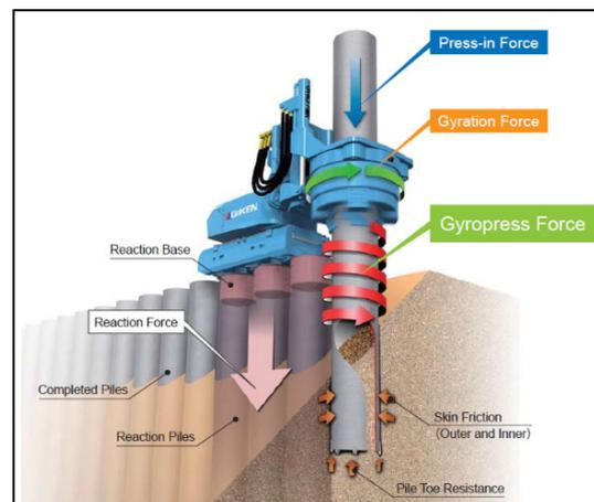
Fig.6 Gyropress Method™<sup>4)</sup>
