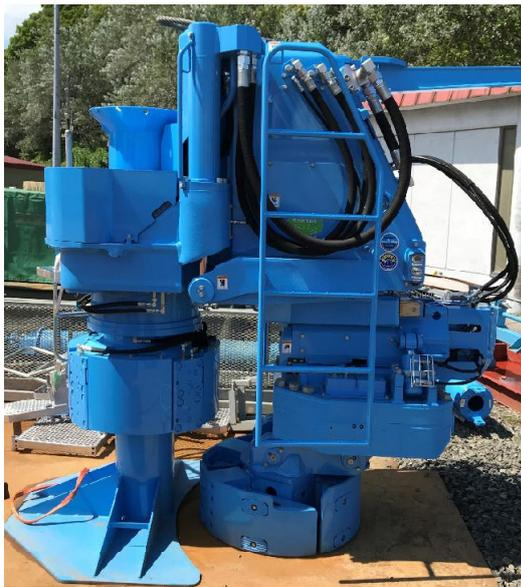
Fig.11 Press-in machine for closure pipe installation
