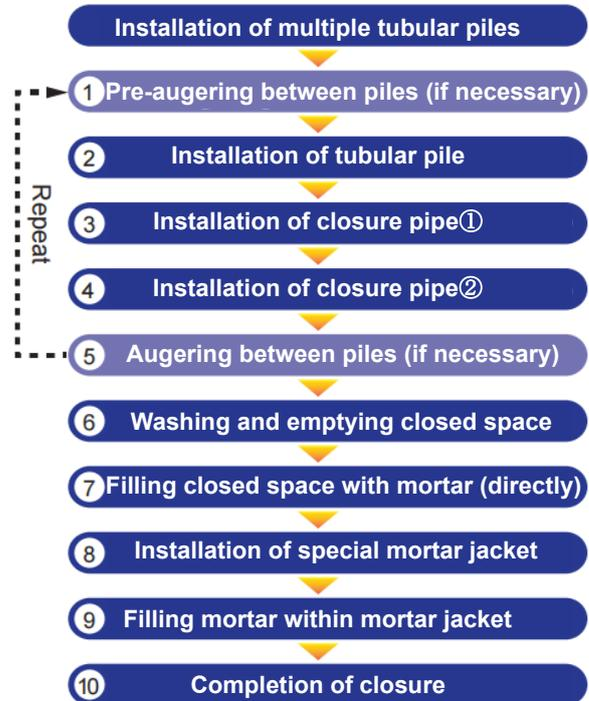
Fig.15 Flowchart of waterproofing method
