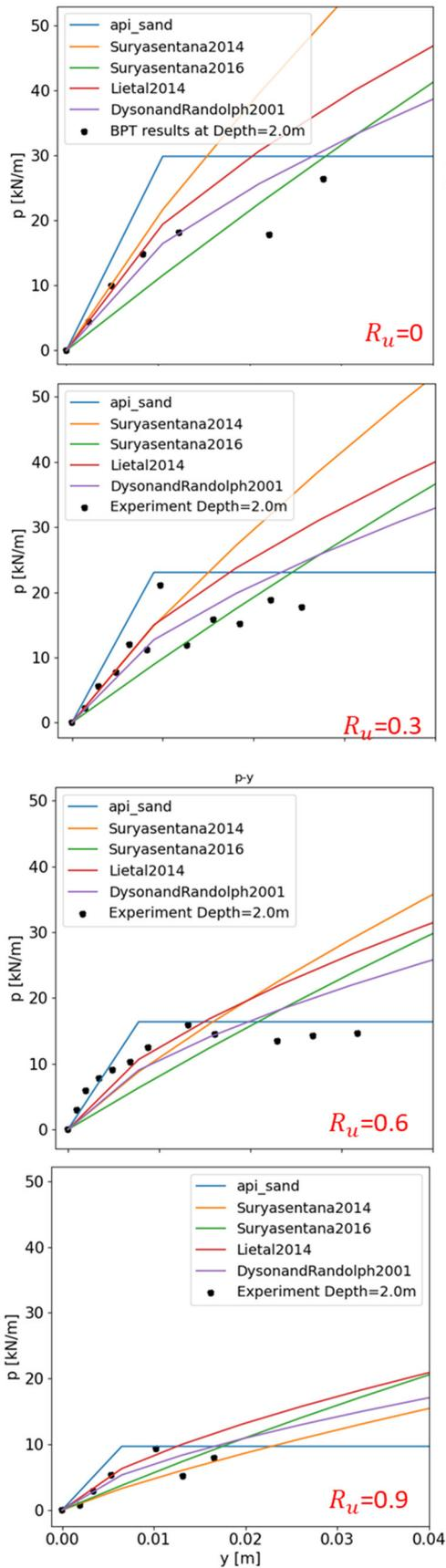
Fig. 10. Simulation of p-y from BPT at depth of 2m
