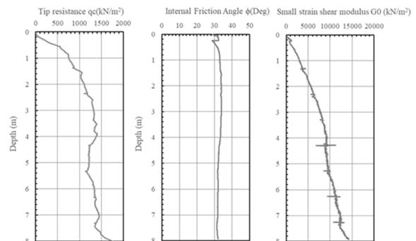
Fig. 3. CPT results, internal friction angle ( $\phi$ ) and the distribution of the small strain shear modulus
