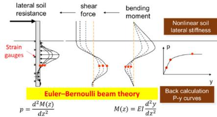
Fig. 5. Derivation of force deflection and p-y curves
