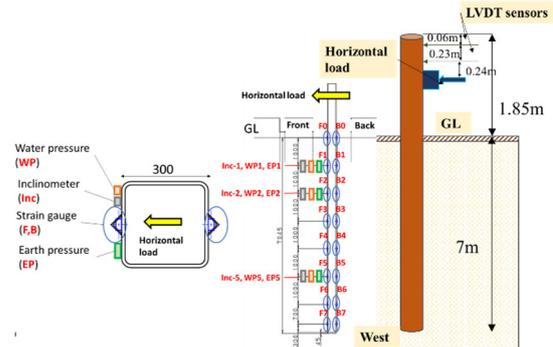
Fig. 2. Horizontal load tests and its instrumentations
