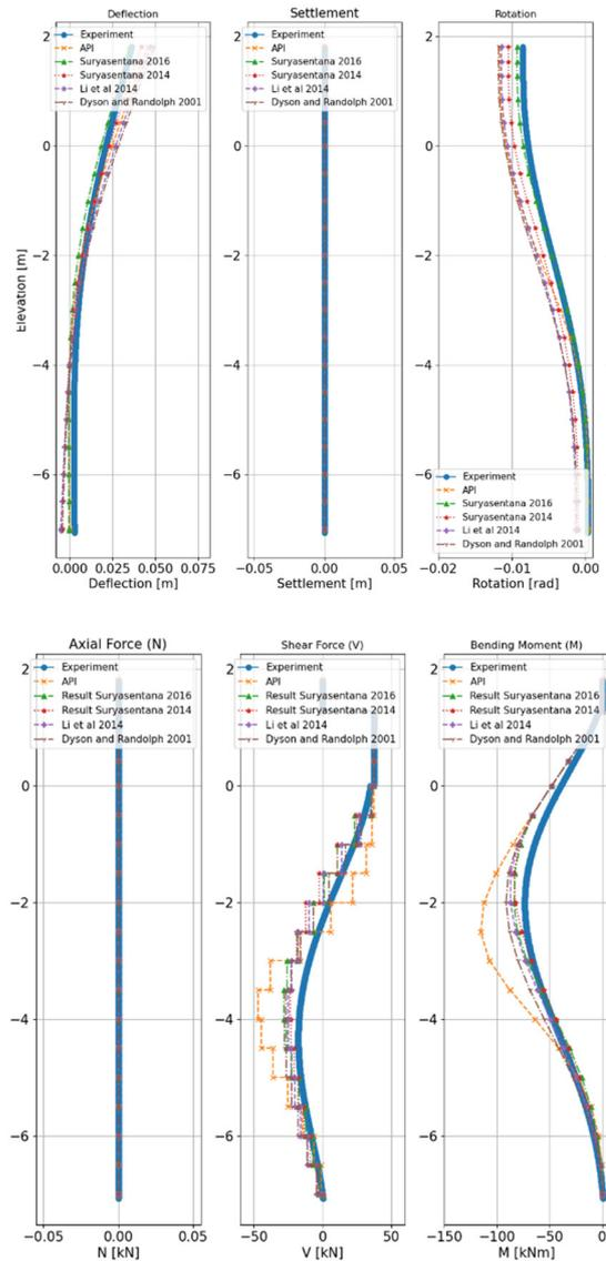
Fig. 11. Predicted pile response using API and CPT based p-y models at  $R_u=0$
