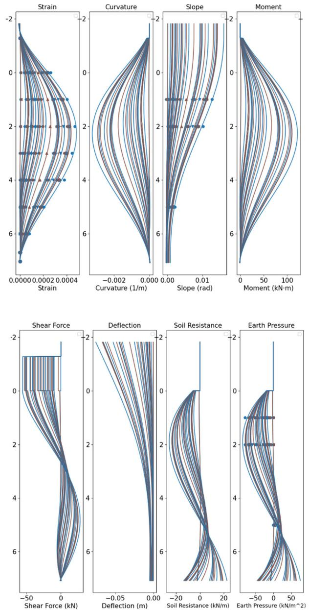
Fig. 7. Measured response of laterally loaded pile at ( $R_u=0$ )
