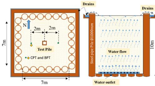
Fig. 1. Schematic view of liquefaction testing apparatus
