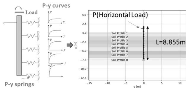
Fig. 4. Schematic diagram of 1D FEM of Laterally loaded pile
