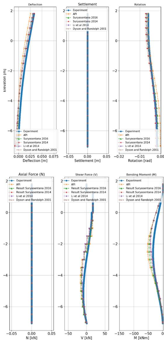
Fig. 12. Predicted pile response using API and CPT based p-y models at  $R_u=0.6$
