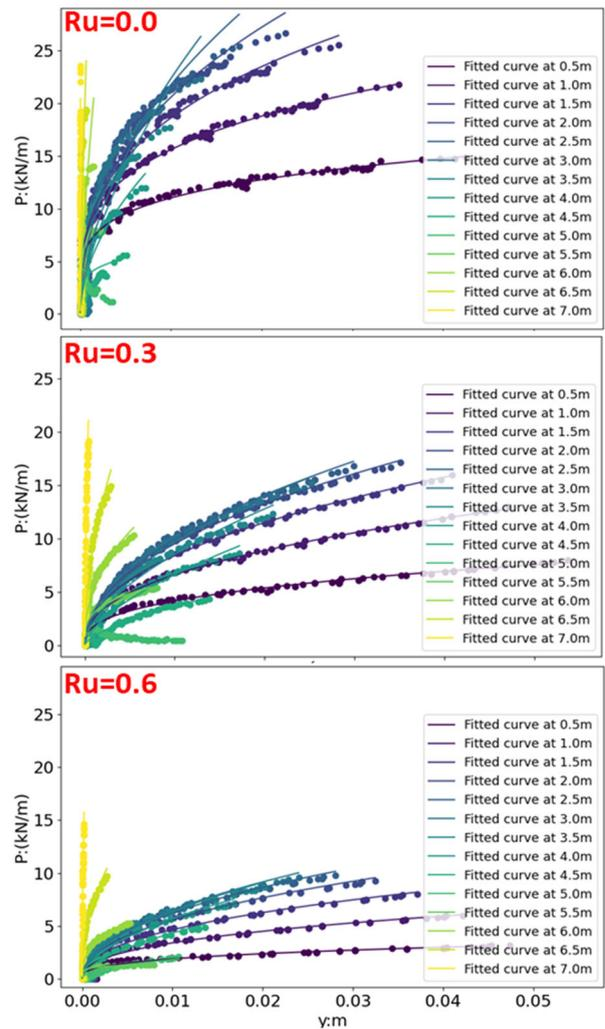
**Fig. 8.** P-y curves back calculated from the results of HLT tests
