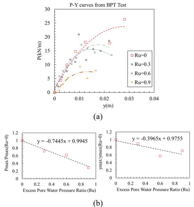
**Fig. 9.** (a) P-y curves (b) P<sub>max</sub> and y<sub>max</sub> correlation
