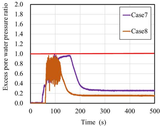
Fig.20 Excess Pore water pressure ratio at P6 (Sheet pile closing method)
