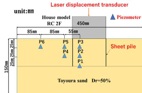
Fig.15 Case7 ; Sheet pile closing method
