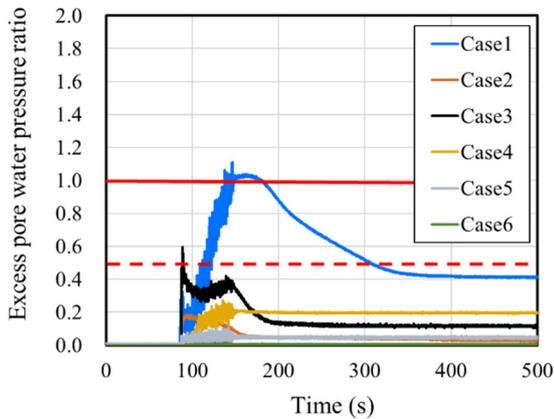
Fig.17 Excess Pore water pressure ratio at P3 (Glass gravel improvement)
