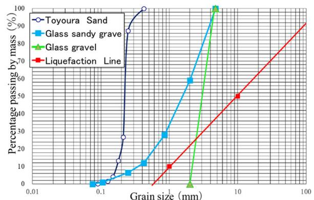
**Fig. 2** Grain size distribution of Glass granulated sand
