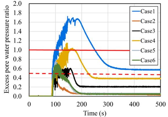
Fig.18 Excess Pore water pressure ratio at P6 (Glass gravel improvement)
