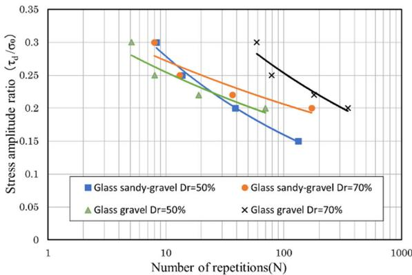
**Fig. 3** Liquefaction resistance of Glass granulated sand
