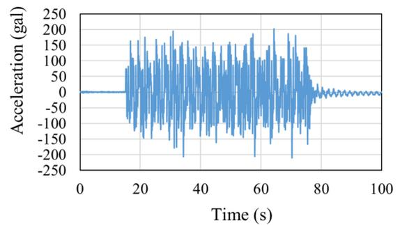
**Fig. 4** Input seismic waves of the shaking table
