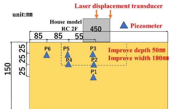
**Fig. 5** Experimental model for the Detached house
