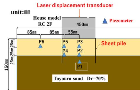
Fig.16 Case8 ; Sheet pile closing method
