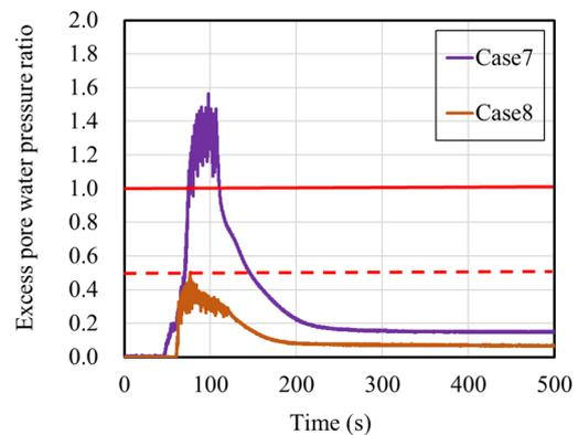
Fig.19 Excess Pore water pressure ratio at P3 (Sheet pile closing method)
