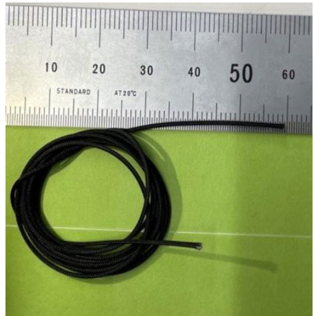
(b) FBG cable protection coating
