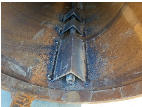
Fig. 8 Pipe guard angles for jet pipe
