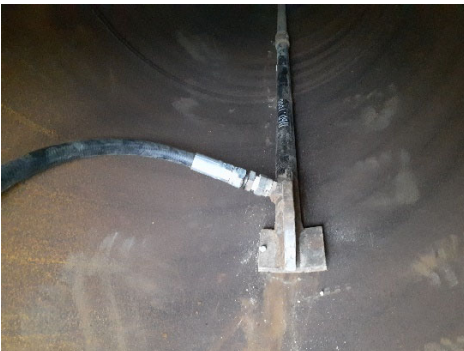
Fig. 7 Pipe stopper equipment
