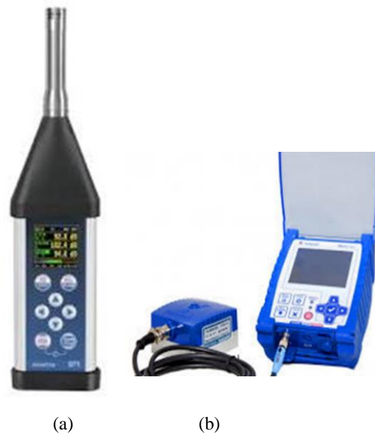
Fig. 7 (a) Svantek 917 noise measurement device, (b) Instanet Micromate vibration monitor and receiver
