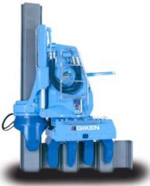
Fig. 2 Press-in piling machine, known as “Silent Piler”
