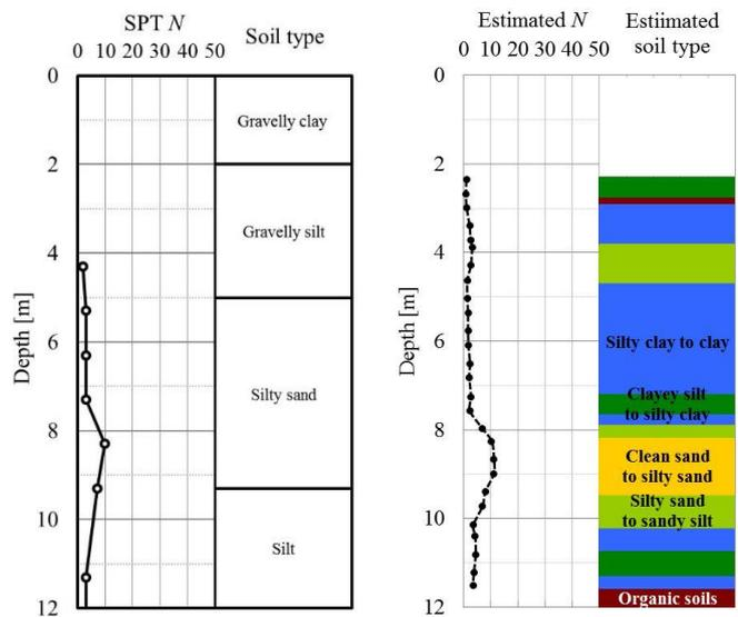
**Fig. 9** Results of SPT and estimation (C11-05).
