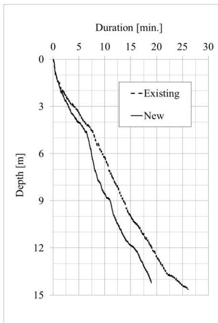
Fig. 6 Duration of a single pre-augering process.
