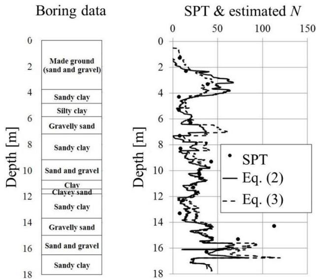
**Fig. 11** Results of SPT and estimation (pre-augering process in press-in with augering).
