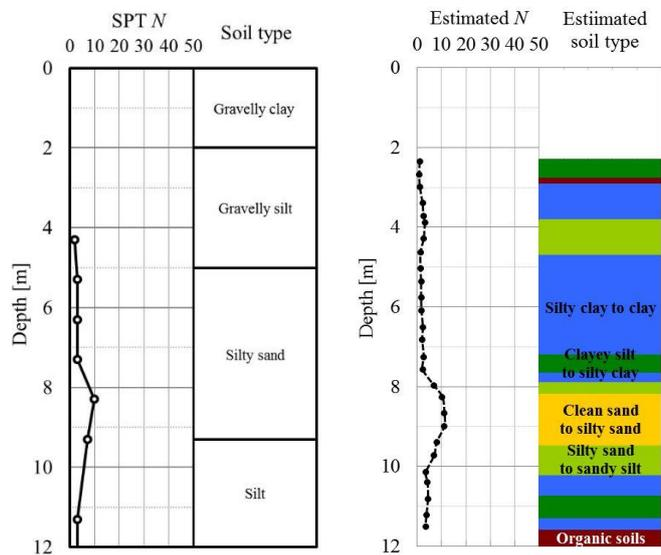
Fig. 9 Results of SPT and estimation (C11-05).
