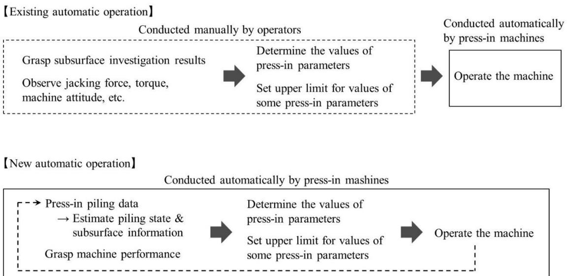
**Fig. 3** Concept of the use of the press-in piling data.
