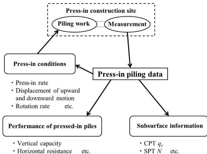
Fig. 2 Concept of the use of the press-in piling data.
