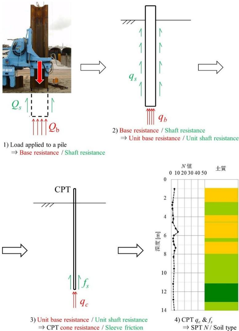
Fig. 7 Estimation process in standard press-in.
