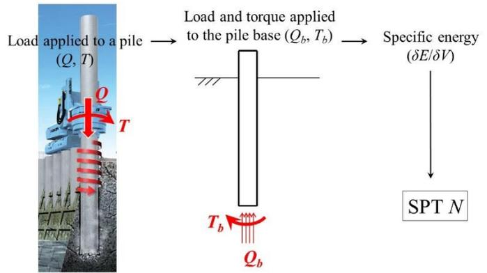
Fig. 8 Estimation process in rotary cutting press-in.
