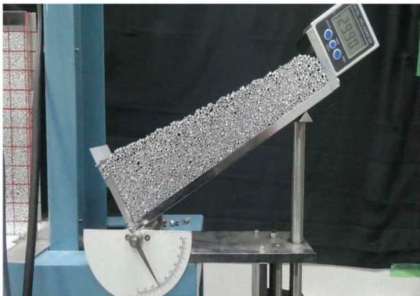
Figure 3. Measurement of internal angle of friction (just after the aluminum rod collapsed).
