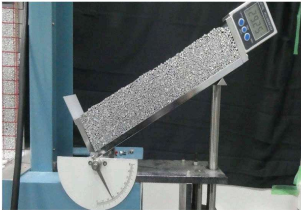
Figure 2. Measurement of internal angle of friction (just before the aluminum rod collapsed).
