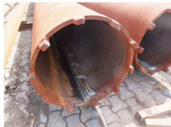
(b) 1000 mm tubular pile with cutter bits
