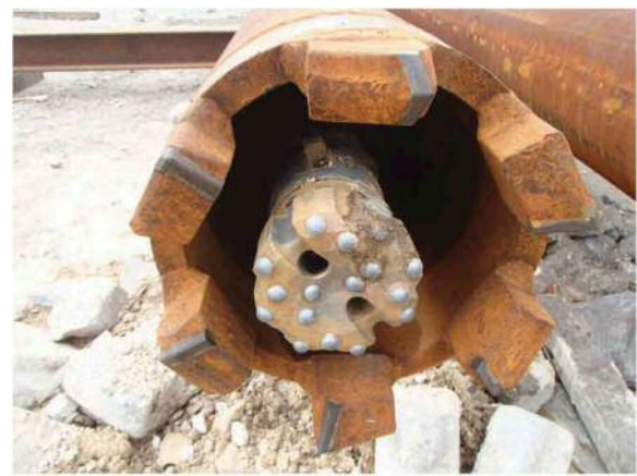
(a) 318.5 mm tubular pile with cutter bits
