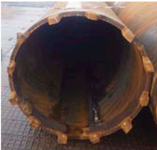
Figure 6. Steel pipe pile with pile toe ring bits.
