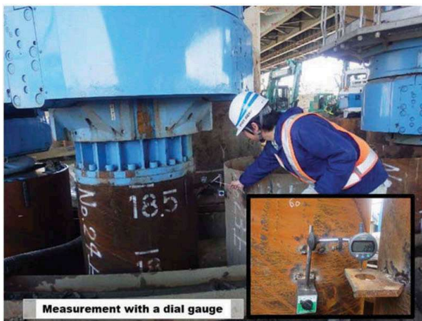
Figure 16. Vertical loading test.
