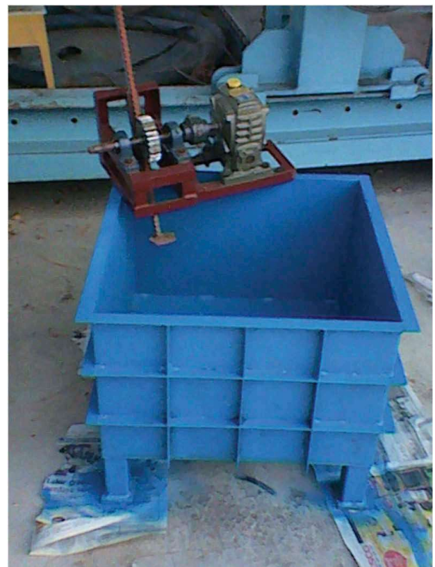
Figure 21. A self-fabricated pile extraction mechanism and test bed.
