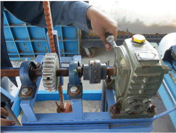
Figure 22. A self-fabricated pile extraction mechanism.
