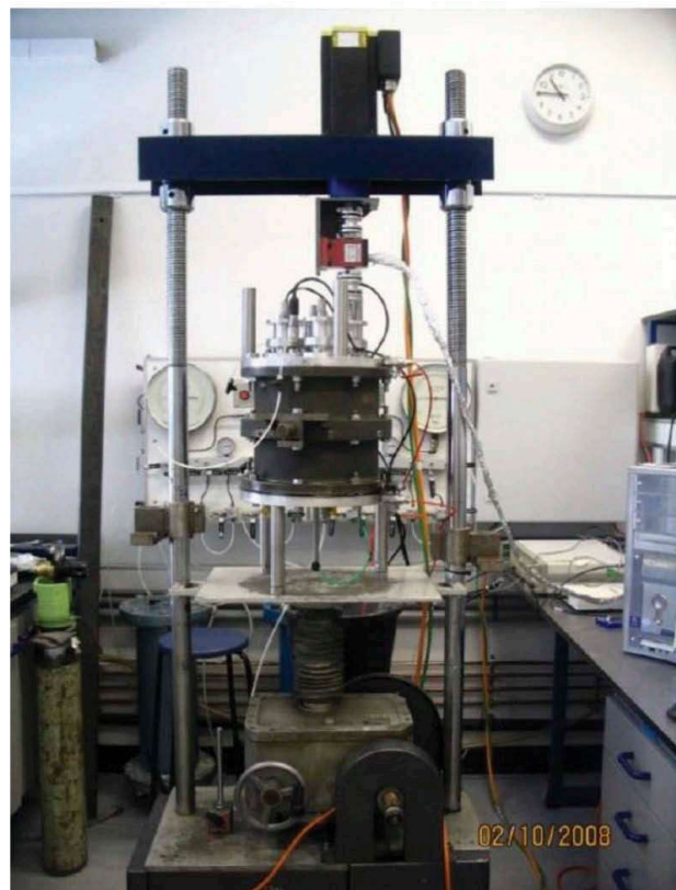
Figure 2. Rowe Cell Vane Shear Apparatus.
