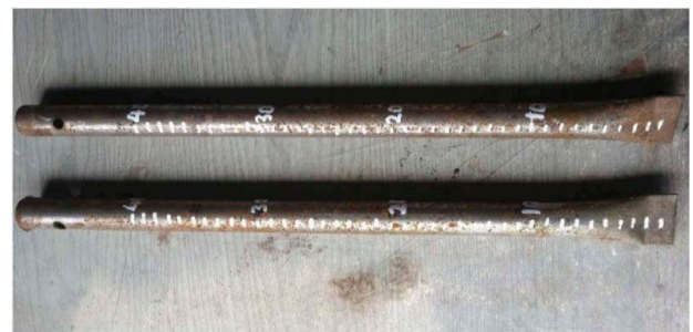
Figure 20. Circular model pipe piles.
