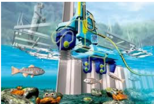
Figure 3 Seabed piling rig ( www.giken.com )
