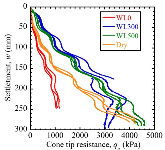
Fig. 5 Results of CPTs in model ground
