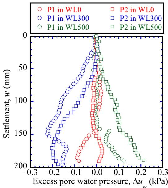
Fig. 8 EPWP-settlement curves during PPTs
