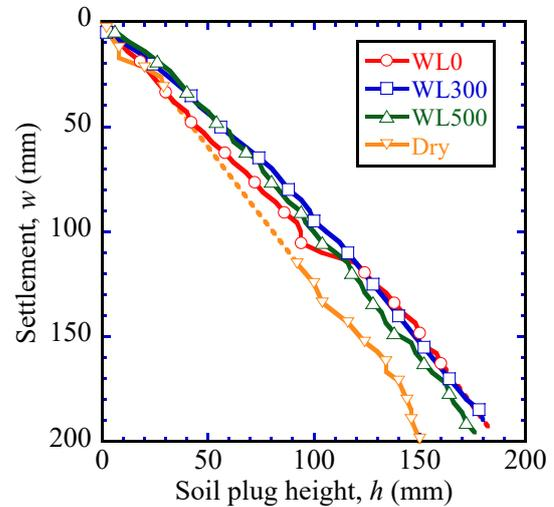
Fig. 7 Soil plug height-settlement curves during PPTs
