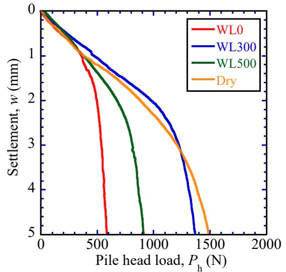
(a) Pile head load vs. settlement
