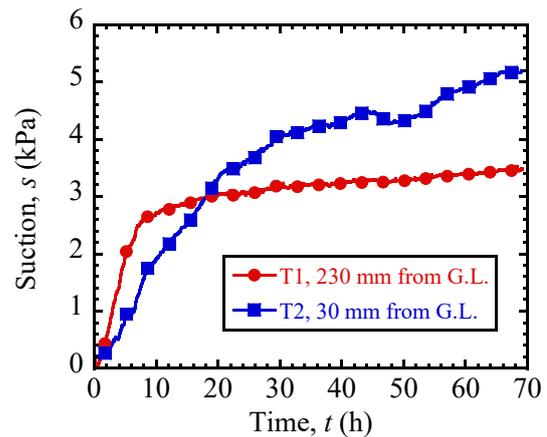
Fig. 4 Changes in suction after moving the water tank (WL=500 mm)
