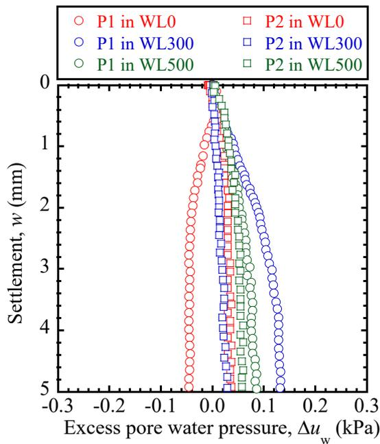
Fig. 10 EPWP-settlement curves during VLTs
