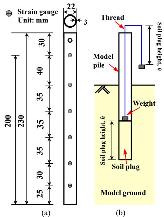
Fig. 2 Model pile: (a) Dimensions and strain gauges; (b) Method for measuring the height of soil plugs
