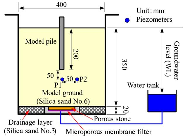
Fig. 1 Schematic diagram of the soil tank
