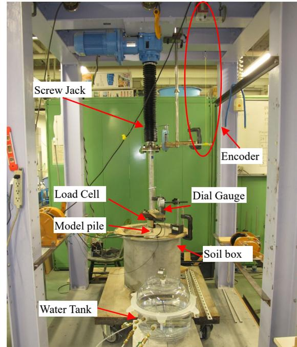
Fig. 3 Experimental set-up
