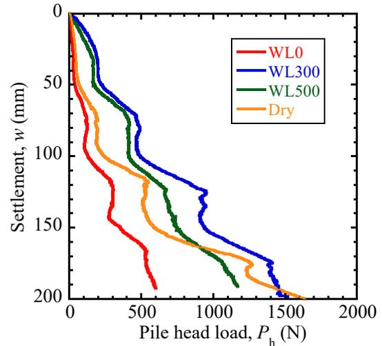
Fig. 6 Load-settlement curves during PPTs
