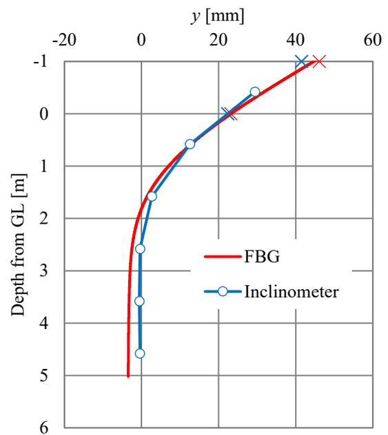
Fig. 15 Comparison about horizontal displacement at  $p=50\text{kN}$
