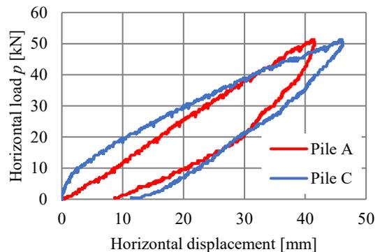
**Fig. 11** Loading test result at loading point
