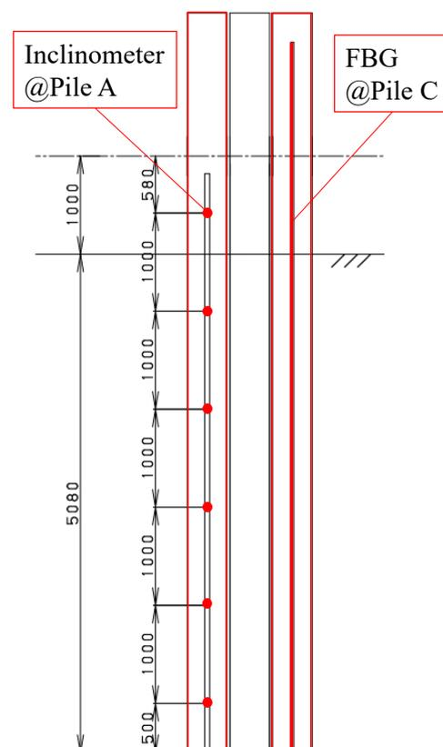
Fig. 4 Measurement points of test pile
