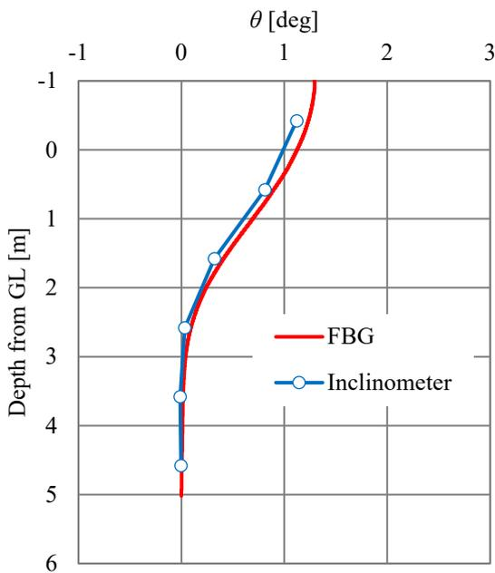
Fig. 14 Comparison about inclination at  $p=50\text{kN}$
