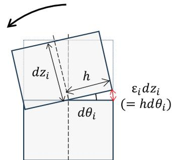
**Fig. 9** Conversion from strain to inclination
