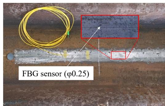
**Fig.7** FBG sensor on test pile
