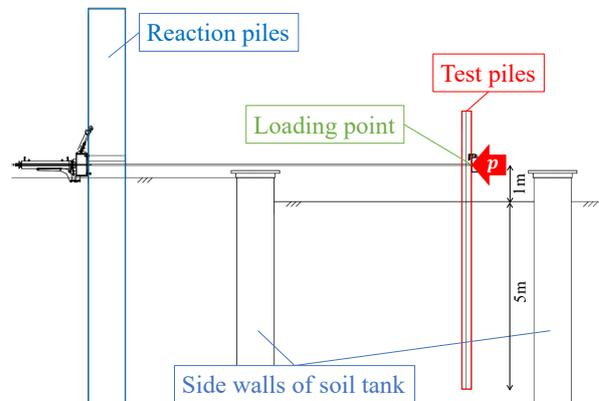
**Fig. 6(b)** Test layout (side view)
