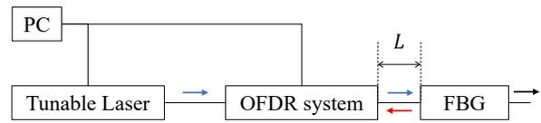
Fig.2 OFDR measurement system
