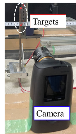
Fig.3 Two red circles were attached at the tip of the pile and their movements were recorded by camera
