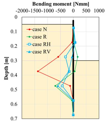
Fig. 9 Incremental bending moment due to excavation
