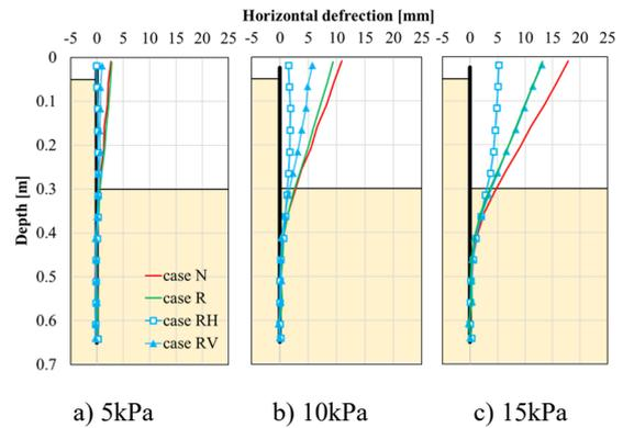
**Fig. 14** Incremental horizontal deflection due to the backside surcharge in service
