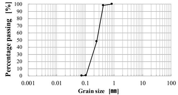
**Fig. 3** Property and grain size accumulation curve of silica sand #6
