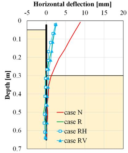
Fig. 8 Incremental horizontal displacement due to excavation method of applying preload needs to be investigated.
