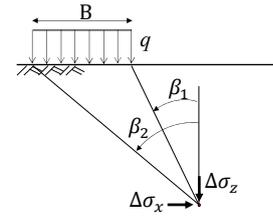
Fig. 7 Stress increases due to surcharge
