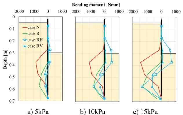
**Fig. 15** Incremental bending moment due to the backside surcharge in service
