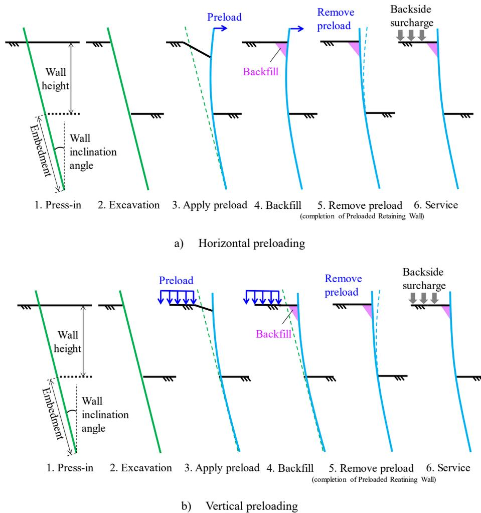
**Fig. 1** Construction procedure of Preloaded Retaining Wall
