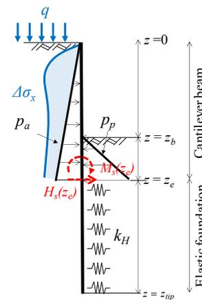
**Fig. 6** Schematic diagram of calculation of deflection due to backside surcharge
