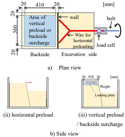
**Fig. 5** Loading methods
