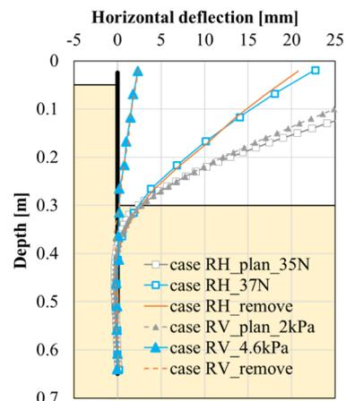
Fig. 11 Incremental wall deflection due to the application and removal of preload
