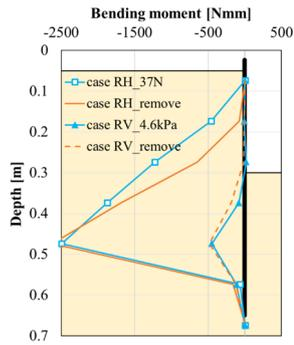
**Fig. 12** Incremental bending moment due to the application and removal of preload
