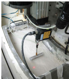
Fig. 13 T-bar penetration test (Almeida et al. 2013)
