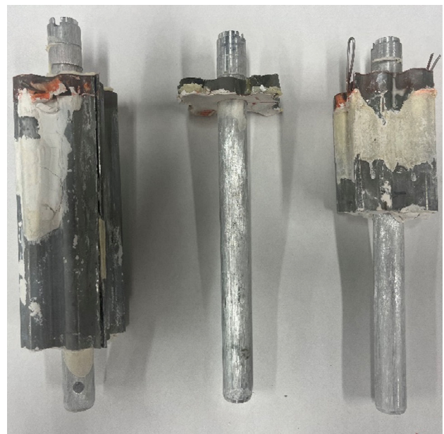
Figure 10 Exhumed foundations after the test
