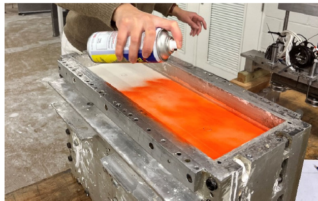
Figure 4 Method of sealing the surface of the clay model
