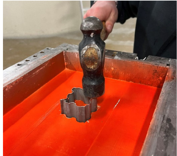
Figure 5 Installing the embedded sheet piled wall
