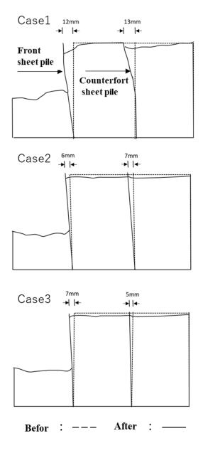
Fig.6 Displacement diagram of the quay before and after the experiment
