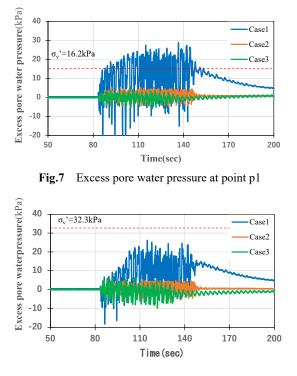
Fig.8 Excess pore water pressure at point p2
