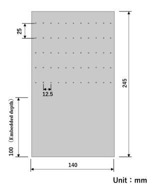
Fig.3 Hole arrangement of permeable steel sheet pile
