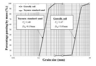
Fig.4 Grain size accumulation curve of the ground material used in the experiment
