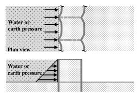
Fig. 7 Actual deflection in the width direction
