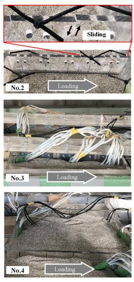
Fig. 12 State of the partition walls at a displacement of 20mm
