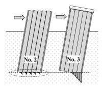
Fig. 18 Expected ground resistances at partition wall base
