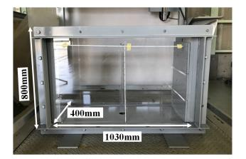
Fig. 3 Soil tank of the 1-g model experiment
