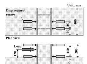
Fig. 8 Layout of the displacement sensors
