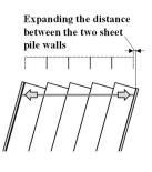
Fig. 10 Cable ties in "unconstrained" case and tension introduced on the cable ties
