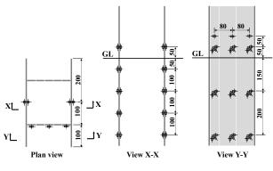
Fig. 9 Layout of strain gauges
