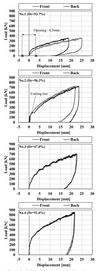
Fig. 11 Load-displacement curves obtained from the test
