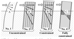
A)Horizontal forces were transmitted through the ground and introduced to the "Front".
