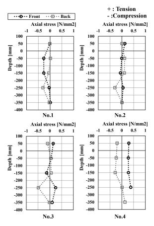
Fig. 14 Axial stress in the double sheet pile walls (when the displacement at GL+0.19m was 20 mm)
