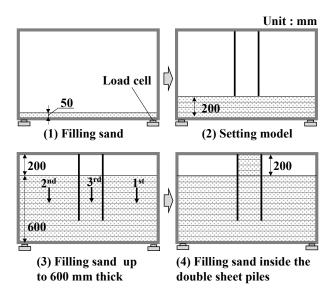
Fig. 5 Preparation of the ground and set up of the model
