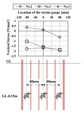
Fig. 15 Vertical stress in the partition walls at GL-0.15m (when the displacement at GL+0.19 m was 20 mm)
