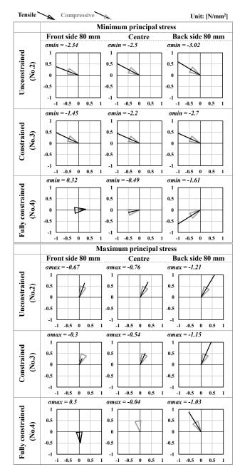
Fig. 16 Minimum and maximum principal stresses in partition walls (when the displacement at GL+0.19m was 20 mm)
