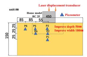
Fig. 5 Experimental model for the Detached house
