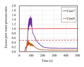
Fig.19 Excess Pore water pressure ratio at P3 (Sheet pile closing method)
