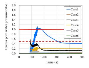
Fig.17 Excess Pore water pressure ratio at P3 (Glass gravel improvement)
