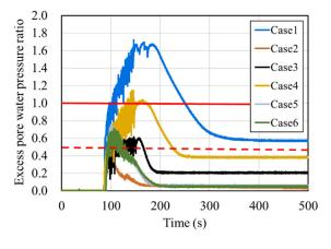
Fig.18 Excess Pore water pressure ratio at P6 (Glass gravel improvement)
