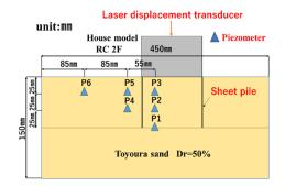
Fig.15 Case7 ; Sheet pile closing method
