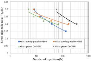
Fig. 3 Liquefaction resistance of Glass granulated sand
