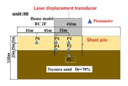
Fig.16 Case8 ; Sheet pile closing method
