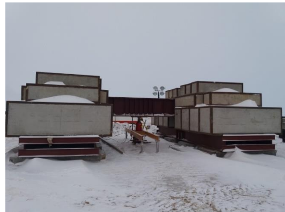
Fig. 1 Vertical static pile test using of SCLT method in seasonally freezing soil ground
