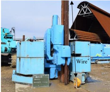
**Fig.6** Situation of press-in piling of zero sheet piles. Wire end was connected to the pile head.
