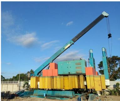
**Fig 3.** Hydraulic static pile driving rig in the Philippines (photo from author)
