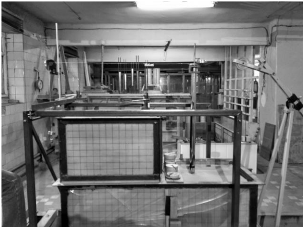
Photo 4. Mooring/fender dolphin model for the second stage of the experiment in the sandy box
