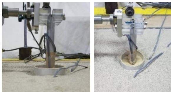
Fig. 12 Conditions after 50 times of cyclic displacement with ring diameter 4D and 3mm pile head cyclic displacement
