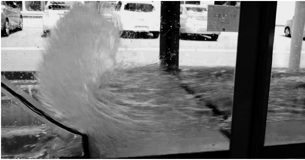
Fig. 5 Model tsunami wave hitting wall
