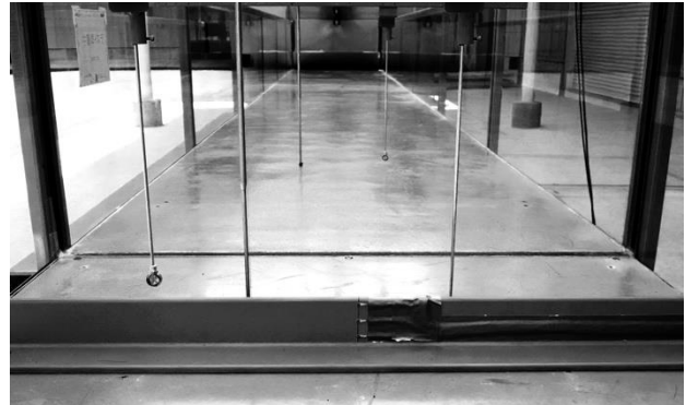
Fig. 3 10cm model wall and wave sensors
