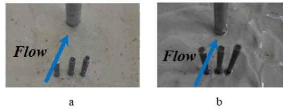
Fig. 5 Photos of model protected by sacrificial piles (a) before and (b) after scour.
