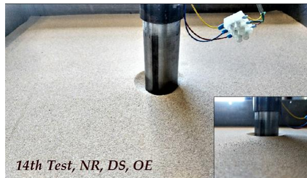
Fig. 11 Surface disturbance for the non-rotated open ended pile installed in dense sand (Pile 1, D=35mm).
