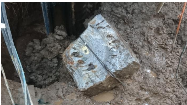
Photo 5. Fragment of granite shows trace of auger head
