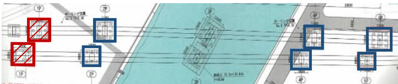
Fig. 7 Adopted seismic reinforcement for foundation (Hatching : Additional pile method, Not hatching : Utilizing Sheet Piles and Soil Improvement)
